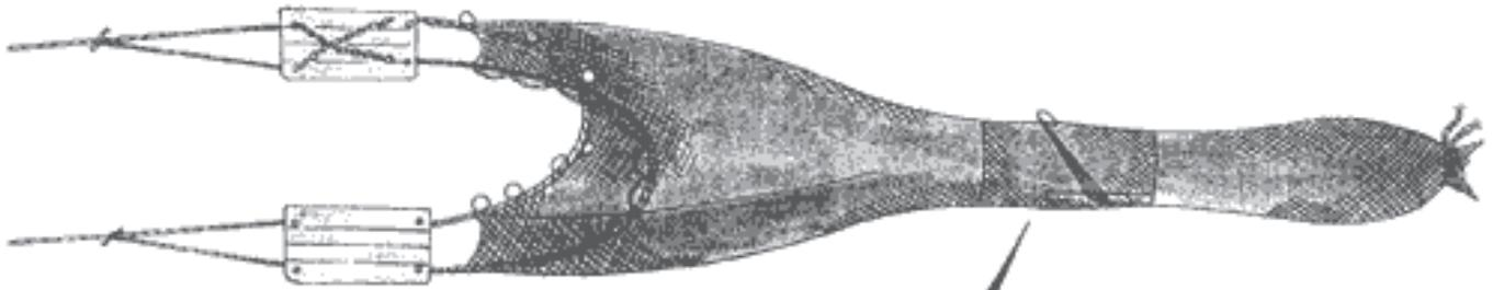
Turtle Excluder Devices are designed to be inserted into trawl fishing nets and allow entrapped sea turtles to easily escape from a trawl net while it is being pulled behind a fishing vessel, as shown in the diagram. The photo below shows a TED frame with the escape flap open.
